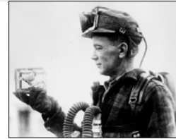
Canaries used to detect CO gas in mines (Hollinger Mine, Ontario, 1928)
